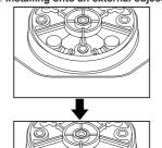
When installing the bracket onto the external object, it has possibility of applying excessive force on the cable due to the lack of space between the cable and the object. f necessary, cut the A part and place the cable to be stable.
