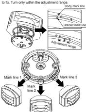
After setting the bracket rotation angle, fix the bracket and laser scanner with the screwdrive
